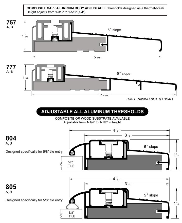
NOTE: Parts 804 & 805 are available in a tall cap version. Order as 904 & 905; which adjust from 1-3/8" to 1-5/8" in height.
