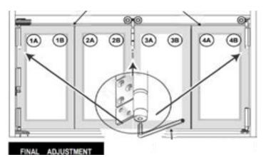
UP AND DOWN ADJUSTMENTS These are located on the top Pivot and any carrier set. Close the door completely to access these adjustments from the exterior using a 5/16" Allen wrench.
