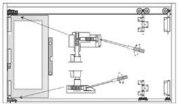
SIDE TO SIDE ADJUSTMENTS These are located only on the Pivot hardware, top and bottom.
