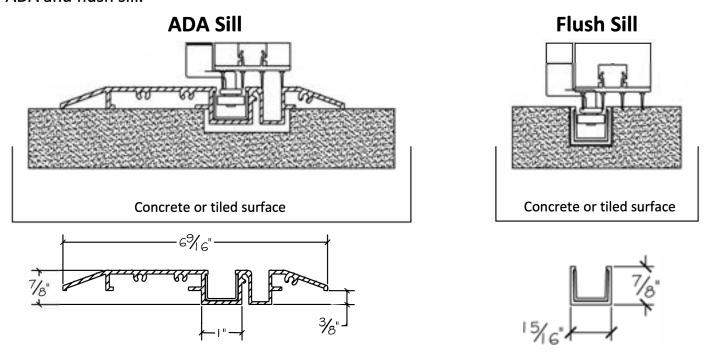
Please note. While the ADA and Flush Sills are very attractive options, it is not intended for all applications. Low or flush sills are not able to withstand air and water intrusion like the weather resistant sills. Your projects exposure, elevation and overhang will determined how this sill performs. It is also important that you include a mop zone adjacent to these doors, when choosing this options.
