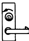
Night latch, key retracts latch bolt. Lever or knob is rigid. Use NL suffix. (Rim cylinder not included)
