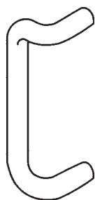
Size: 11" Round: 1" CTC: 10" Clearance: 2-1/4" BHMA: J402 ADA compliant
